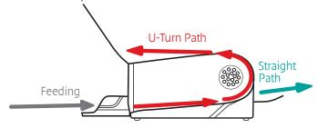
An added straight-through paper path enables smooth scanning of plastic cards and thick documents.
